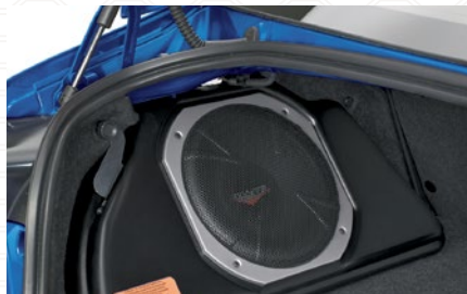
10-inch Powered Subwoofer. Provides powerful, deep bass, and also assists in clean sound reproduction from all vehicle speakers. This is achieved by its integrated 100W amplifier and a passive crossover network. Manufactured for Subaru of America by Kicker®.
