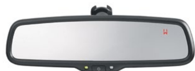
Auto-dimming Mirror with Compass. Mirror automatically darkens when headlights are detected from behind the vehicle. Features an electronic compass with a red transfective display that projects the current direction onto the mirror's surface.
